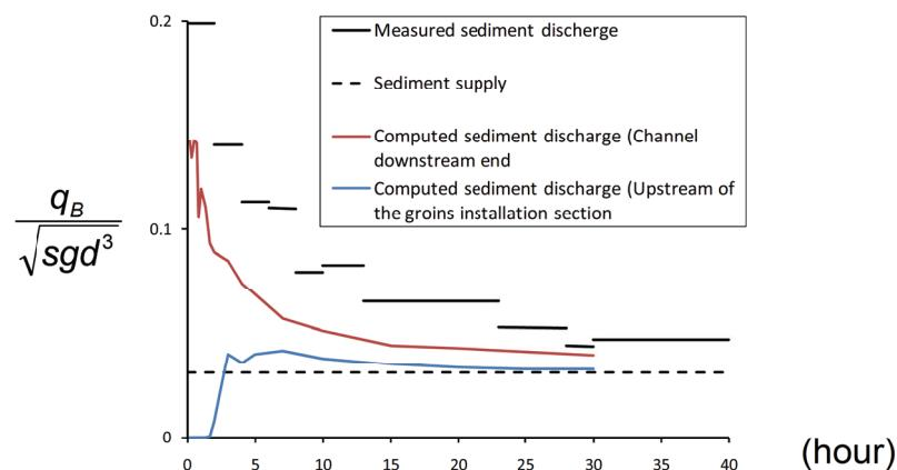
**Figure 4 Comparisons of temporal changes in sediment discharge between the measurement (Fukuoka *et al.*, 1998) and the computation by present method.**
