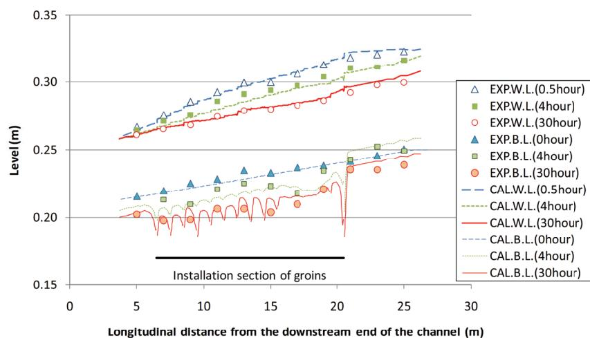
**Figure 3 Comparisons of temporal changes in longitudinal water and bed level between the measurement (Fukuoka *et al.*, 1998) and the computation by present method.**
