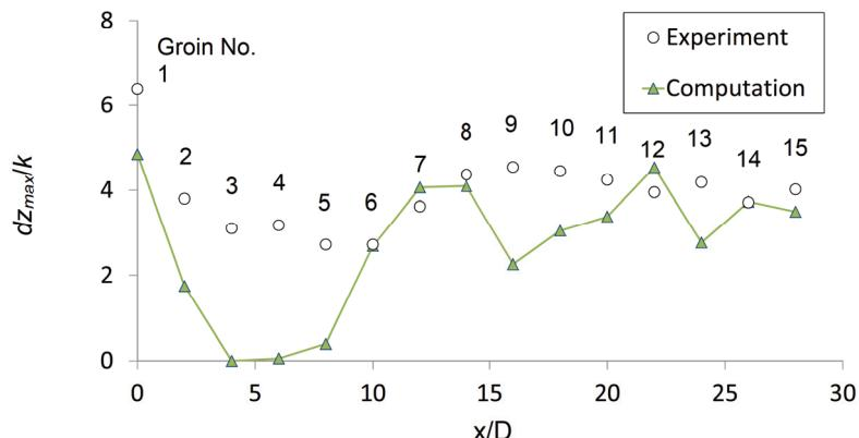
**Figure 8 Longitudinal distribution of maximum scour depth around groins**
