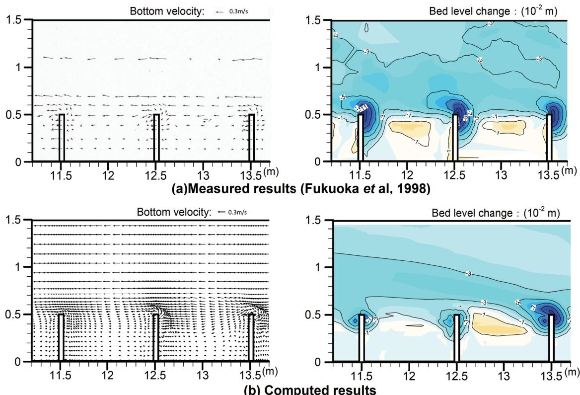
**Figure 6** Bottom velocity distributions and bed topographies in the midstream of the installation section by the measurement and the computation at the dynamic equilibrium stage.
