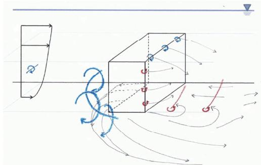
**Figure 7 Flow structures around a submerged groin.**
