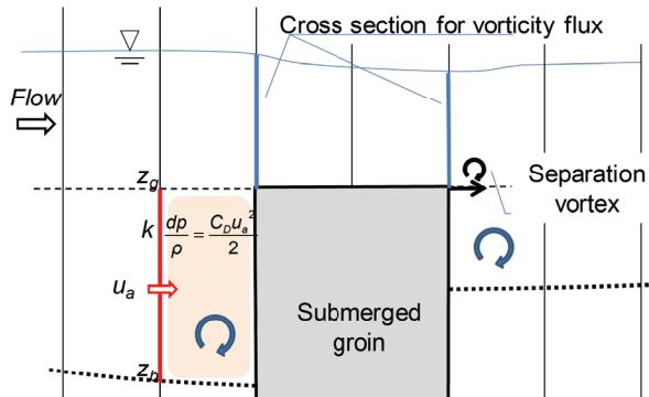
Figure 2 Evaluation method of flow and vortex motion around a submerged groin.
