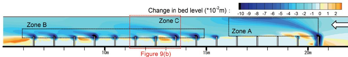
**Figure 5** Computed bed topography in the channel at the dynamic equilibrium stage.
