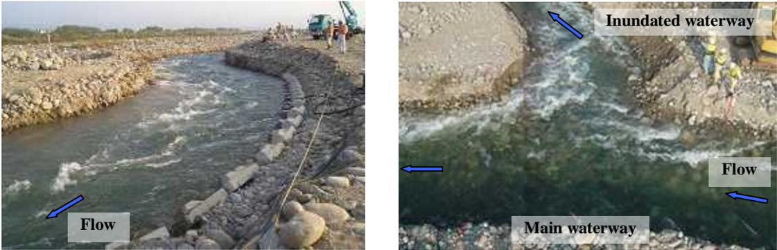
Figure 2. Photograph of the experimental way and inundated water after levee-breach
