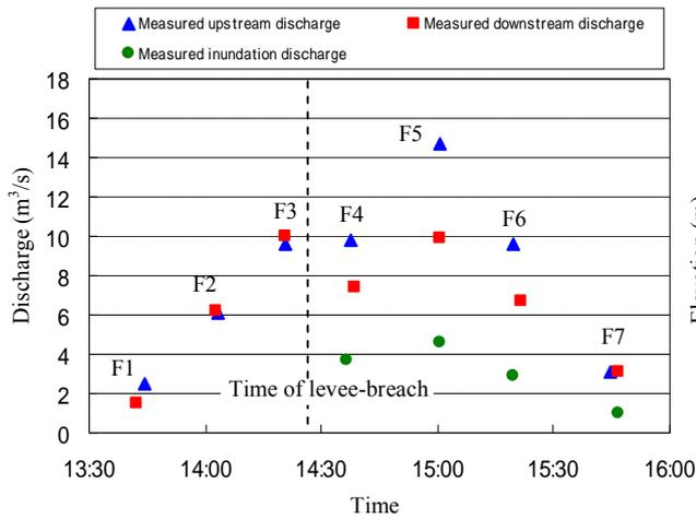
Figure 3. Temporal change in discharge in the experiment
