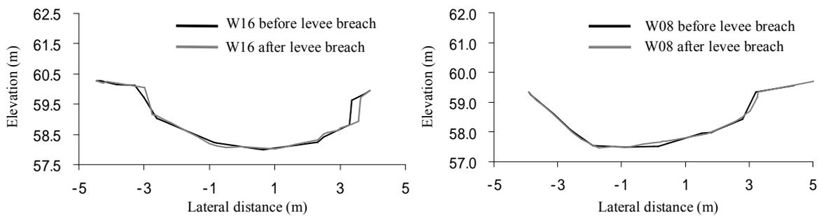
Figure 7. Cross-sectional shape of breach point neighborhood
