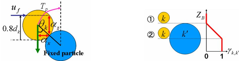
(a) Concept of the pick up particle (b) Calculation method of  $\gamma_{k,k'}$
