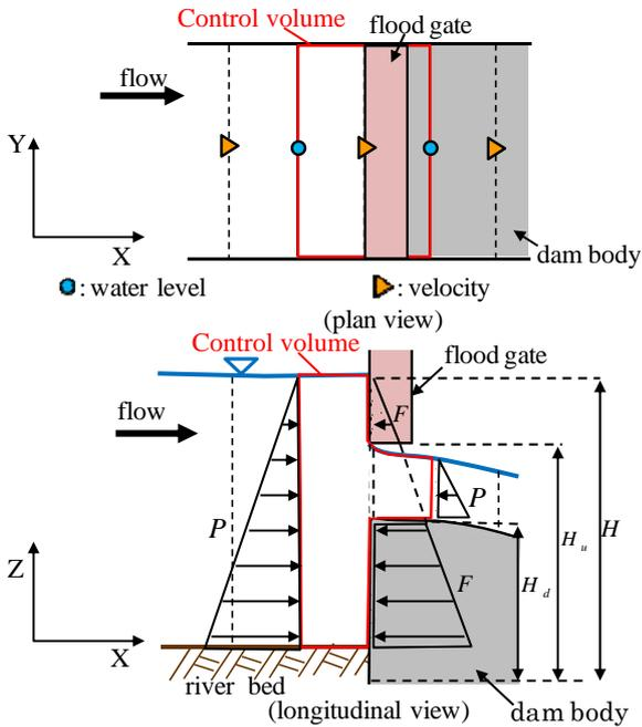
**Fig.8 Concept of analysis for flow over the dam.**
