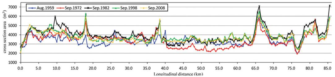
Figure 11. Changes in cross section area.
