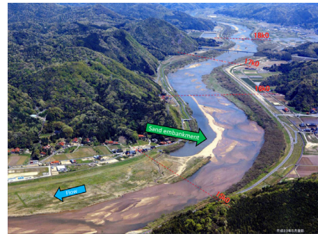
Figure 3. Sand embankment in the main channel.
