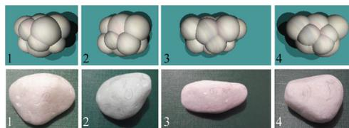
Figure 1. Shapes of model particles and real gravel particles.
