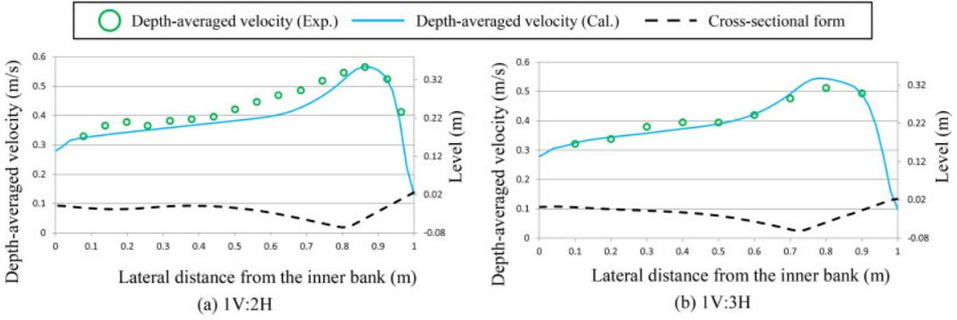
Figure 4. Comparisons of the depth-averaged velocity distributions along the cross-section between the experiments and calculations.
