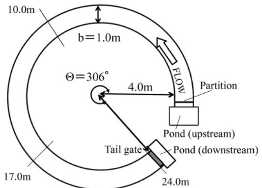
Figure 1. Plan form of the flume.
