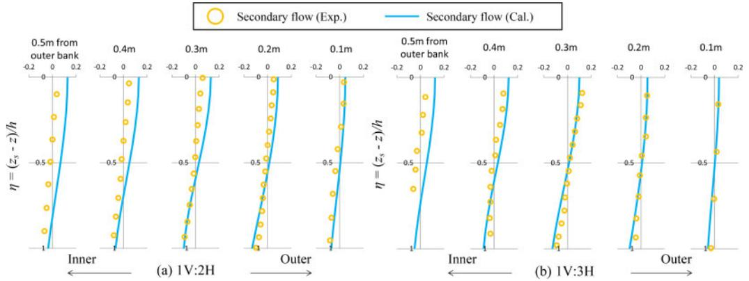
Figure 6. Comparisons of vertical distributions of the secondary flow/cross sectional average velocity between the experiments and calculations. ( $\eta = 0$  : Water surface,  $\eta = 1$  : Bed surface).
