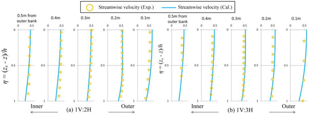
Figure 5. Comparisons of vertical distributions of the streamwise velocity (m/s) between the experiments and calculations. ( $\eta = 0$  : Water surface,  $\eta = 1$  : Bed surface).
