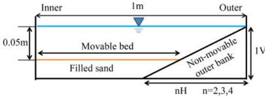
Figure 2. Initial cross-sectional form of flume.
