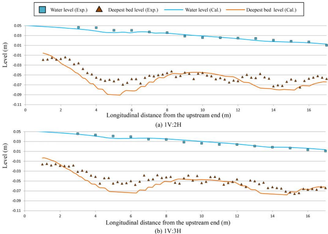
Figure 3. Comparisons of longitudinal water surface profiles and deepest level of channels bed between the experiments (Fukuoka et al. 1995) and the calculation results.
