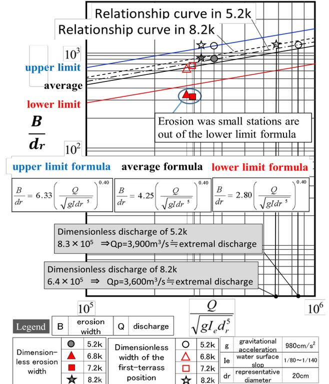
Fig. 5 Correlation of dimensionless erosion width to dimensionless
