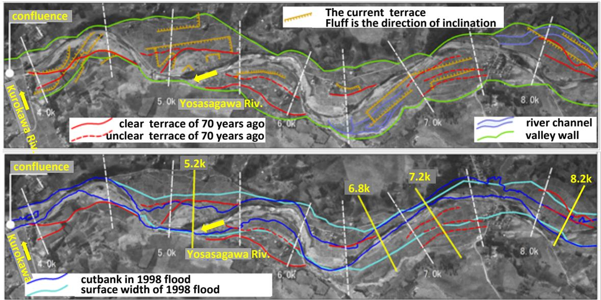
Fig. 3 Erosion width of the 1998 flood、 Step position by the 70-year-old aerial photograph interpretation
