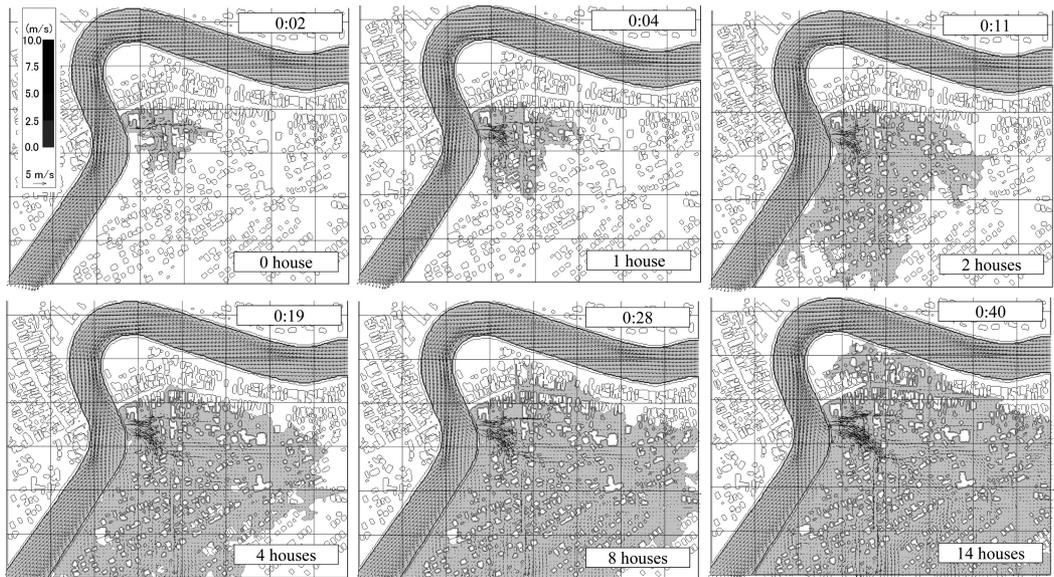
Figure 7. Calculation results of velocity vector, inundated district and total number of houses to be swept away immediately after dyke break (from 2 minutes to 40 minutes after dyke break).
