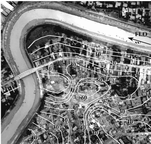
Photo 2. Floodplain damaged and contours of sediment deposition height (unit: cm).
