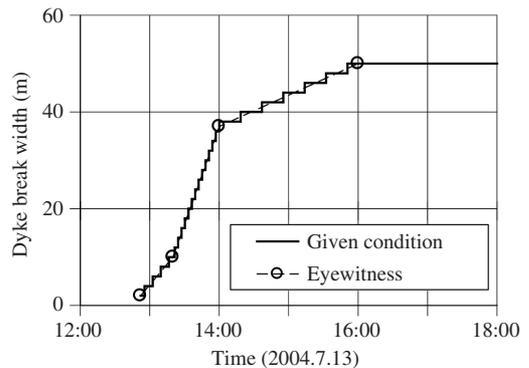
Figure 2. Dyke break width of eyewitness report and given condition in the calculation.
