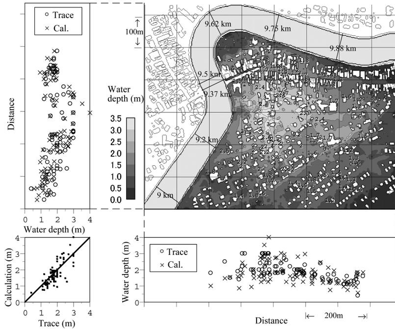
Figure 6. Trace water depth in floodplain and calculated maximum water depth (at 3 hours and 14 minutes after dyke break).
