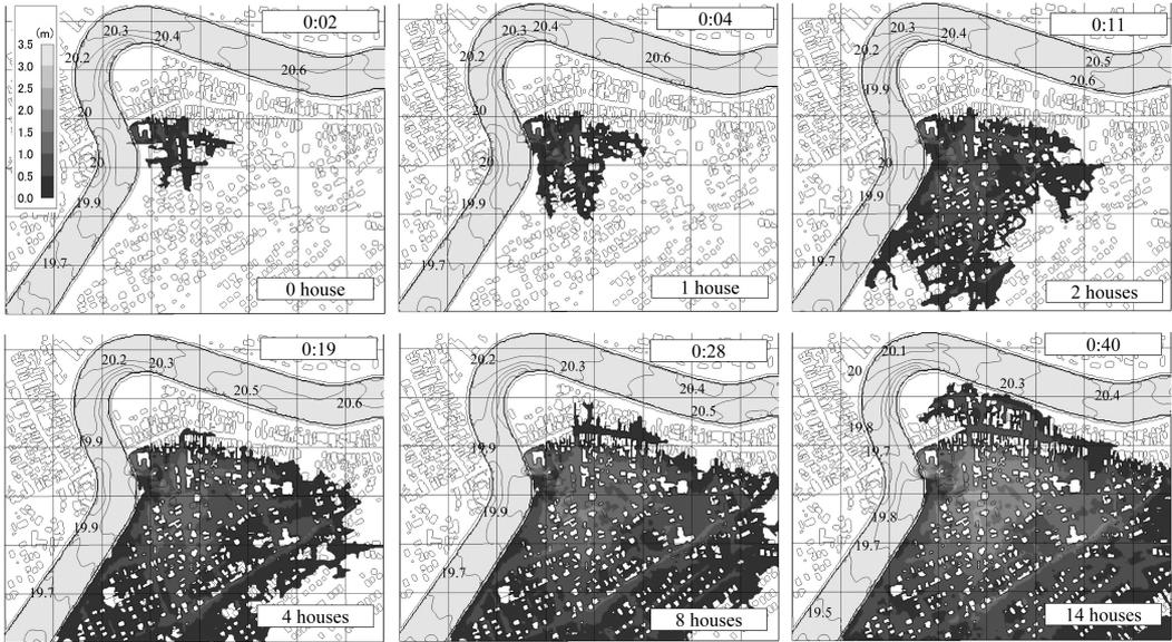
Figure 8. Calculation results of water level in the river channel, water depth in floodplain and total number of houses to be swept away immediately after dyke break (from 2 minutes to 40 minutes after dyke break)
