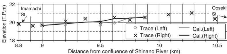
Figure 5. Trace water level on left and right dyke and maximum calculated water level.
