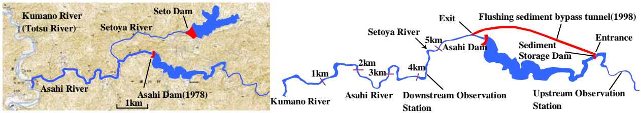
Figure 1. (Left) Asahi River Basin (Right) Plan View of the Flushing Bypass Tunnel
